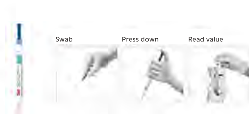
ATP bioluminescence swab testing system operational procedures
